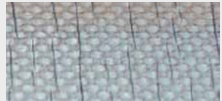
Rubber after running 1000 hours**
