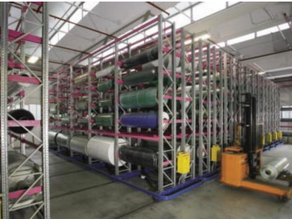
MAGAZZINO SEMOVENTE ROTOLI AUTOMATIC STORING AND SORTING OF ROLLS
