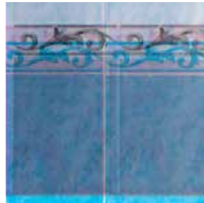
Printing flaws due to irregular belt feed
