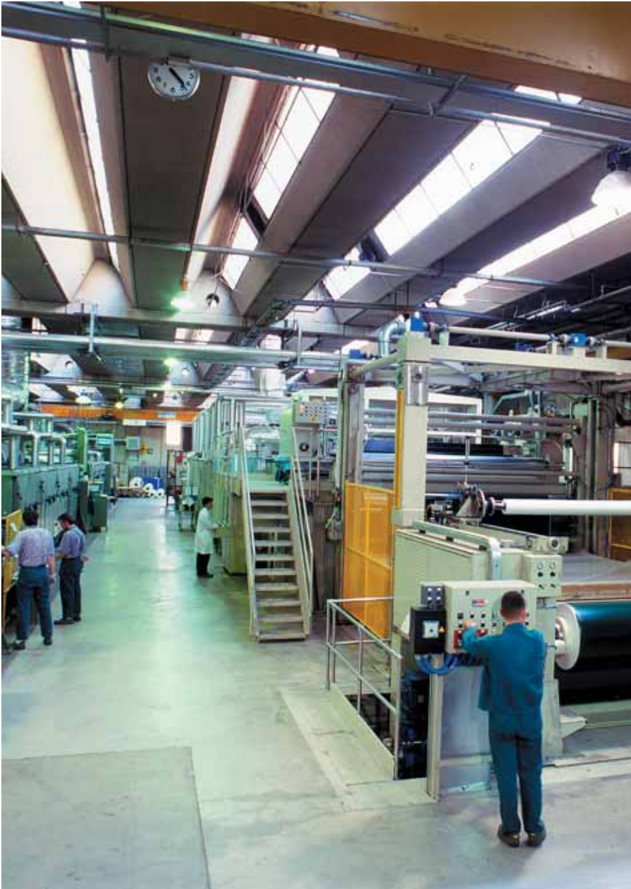
Spreading lines for conveyor belts.
