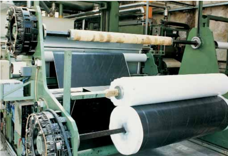
1. Continuous vulcanization line for rubberized rolls in an image from the 1970s. 2. Winder of a PVC belt spreader line.
