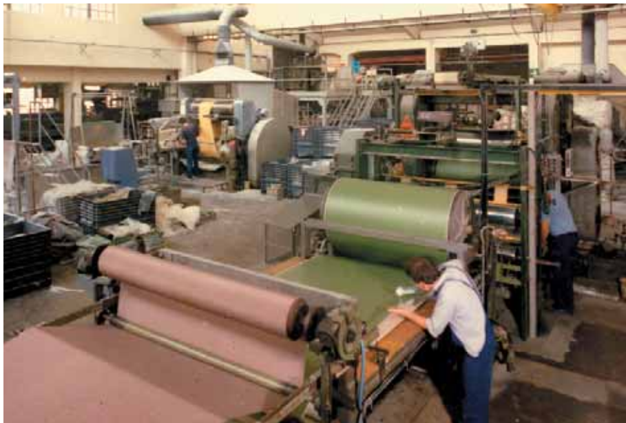
The new calendering lines for rubber conveyor belts.
