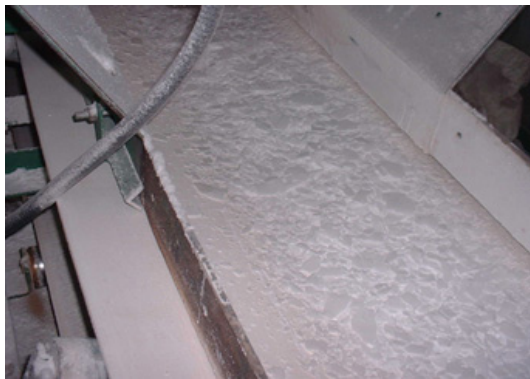
ESPOT 20CC troughed conveyance of chemical product.
