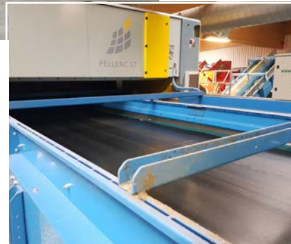
Breda 21UFMT-BK in sorting system with a speed of +4m/s.
